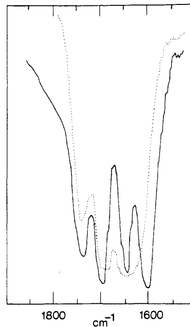
Figure 4. Carbonyl regions of the infrared spectra (KBr) of t -Boc-L-Pro-L-Pro-OH (dotted line) and t -Boc-L-Pro-L-Pro-D-Pro-OH (solid line). In one spectrum recorded as a fluorolube mull, the amide I region of t -Boc-D-Pro-D-Pro-D-Pro-OH could be resolved into two bands occurring at 1653 and 1637 \text{cm}^{-1} .
